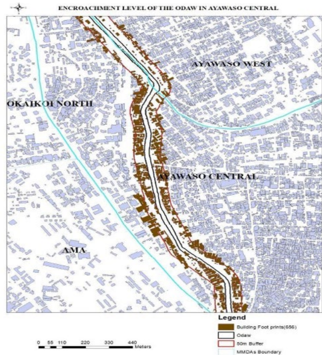
Figure 4: Maps constructed from LiDAR images containing buildings that had encroached the 50-metre buffer zone of the Odaw channel.
