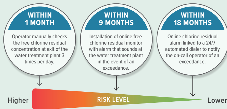
Example of a progressive improvement approach for strengthening chlorine monitoring at a water treatment plant
