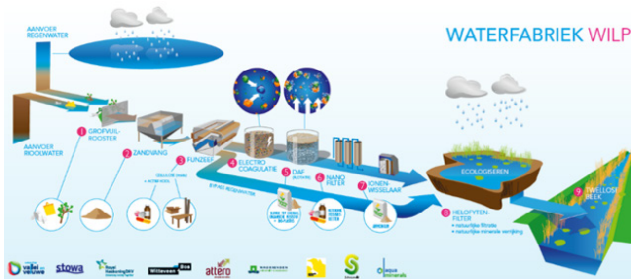
Figure 3.1 Schematic representation of the original rural application of the Water & Resource Refinery.
