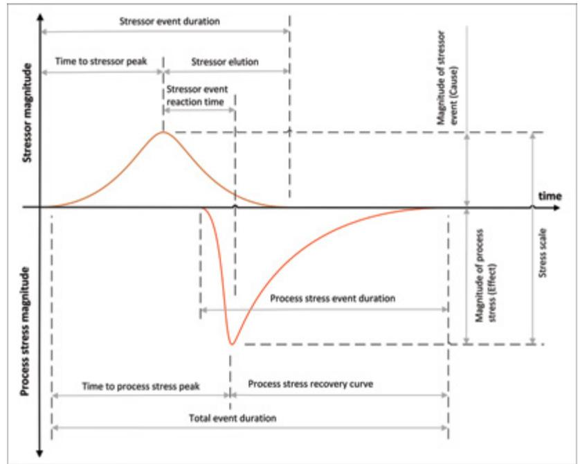
Figure 3.11 Dynamic resilience diagram showing the separation of stressors and process stresses.
