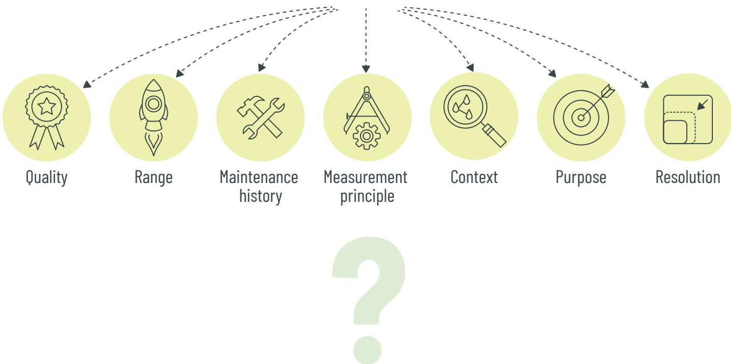
*Figure 1. Can we interpret the provided measurement equal to 42.0? We need to know a lot more to evaluate the information contained in sensor signals. The kind of descriptive data we need for interpretation is known as “meta-data” and includes the purpose of measurement, the measurement principle, the temporal and measurement resolution, sensor maintenance history, indicators of signal quality, and the spatial and temporal context of the measurement.*
