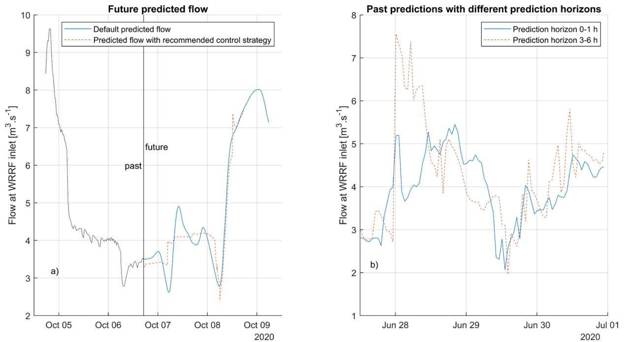
Figure 3. a) Example of model predictions for influent flow to the WRRF using the default control strategy (solid line) and the recommended control strategy suggested by the model (dashed line); b) Example of past model predictions with different prediction horizons (0-1 hours and 3-6 hours).
