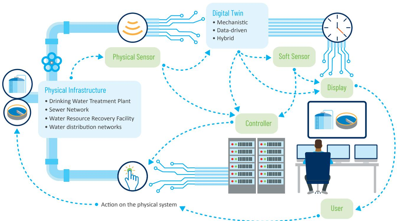
Figure 1. Basic structure of a digital twin application. Elements in blue are basic elements needed for implementation of a digital twin, while elements in green are complementary to the digital twin, ultimately to enable an action on the physical system.
