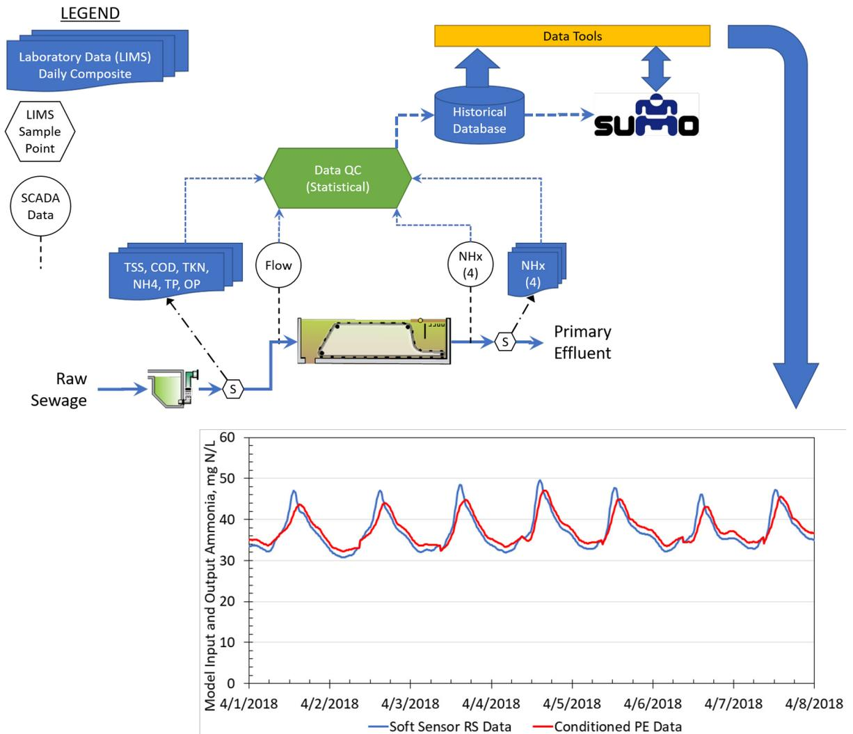
Figure 5: Data flow schematic within digital twin for influent load development for the influent “soft sensor”
