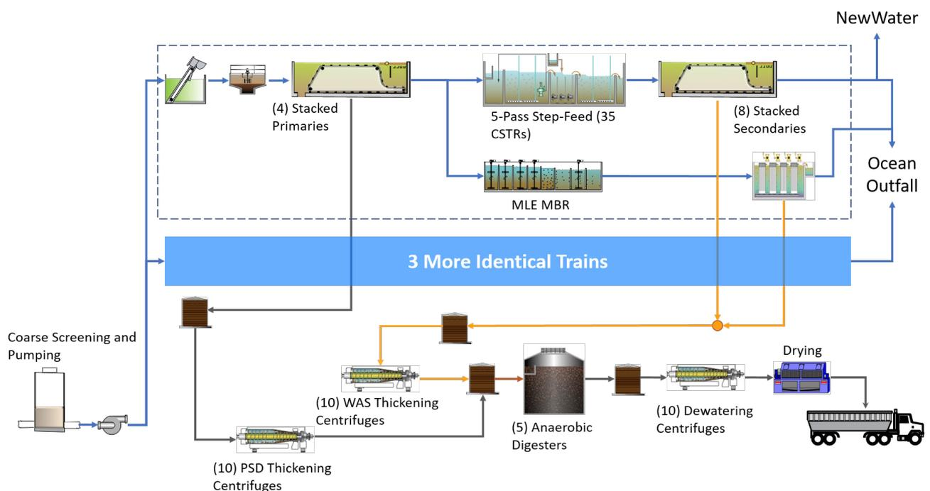
Figure 4. Process flow diagram of Changi WRP and scope of digital twin simulation (inside dashed line). The digital twin includes the four water treatment trains.
