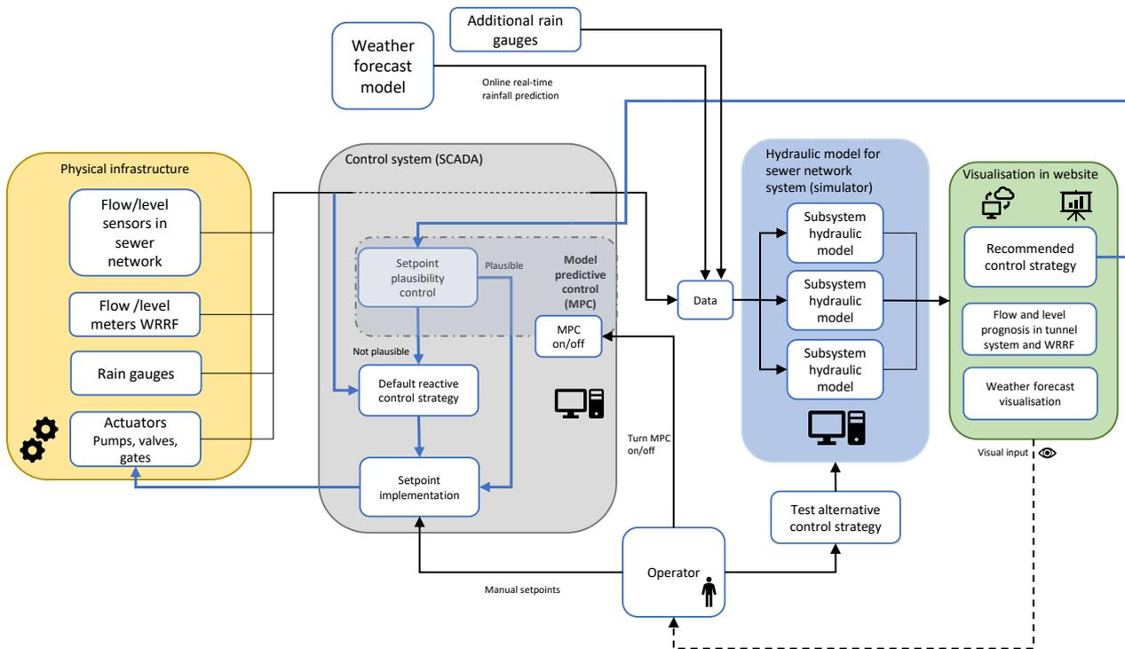
Figure 2. Sewer network digital twin structure and components in the current implementation as well as with model predictive control (work is now underway with the goal of implementing full real-time model predictive control).
