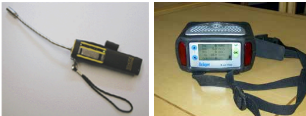
Figure 4. Leak detection instruments. An instrument with semiconductor sensor is shown on the left, and one with a catalytic sensor is shown on the right.
